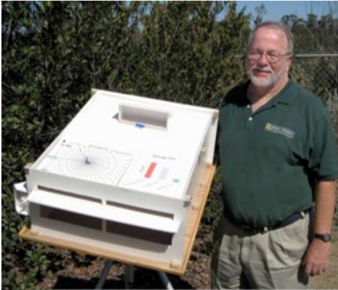
After review by instructor, TA or other teams the daylighting design is created in foam core. The easiest method is to have the back three walls mounted on the solar simulator - students bring south wall and roof. This can have a digital camera port installed on the side near the front (see photo). The students mount their roof and south wall with clips or painters masking tape. They then take exterior and interior pictures hourly from 9 AM - 3 PM on January 21 and September 21.
