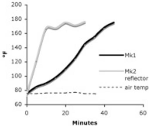
Measure temperature at 5-10 minute intervals, including air temperature.
